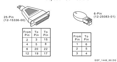
Figure 2-2 VT420 Rear Connector Panel and Loopback Connectors
