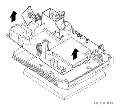
To install the terminal board assembly, reverse the installation steps. If you need to adjust the video display, refer to Chapter 4.
