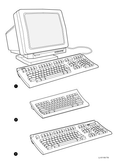
Figure 2–1 VT420 Video Terminal with Keyboards
