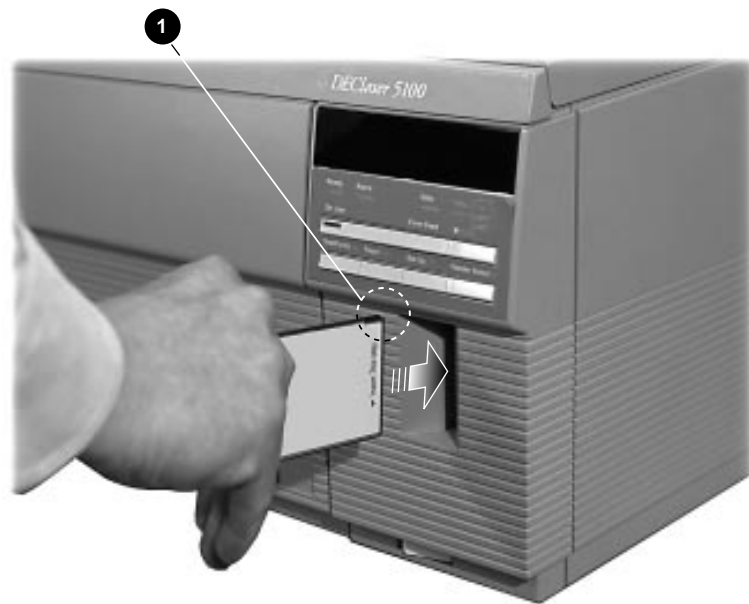
Figure 1–10 Font Cartridge Installation
